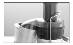
Place both hands on either side of the safety locking arm and pull back and lift over the grooves on either side of the juicing cover.
